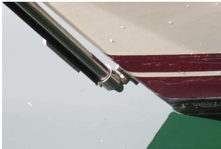
The pivoting hinge mounted to the hull
